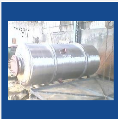
SS Vertical Storage Tank
