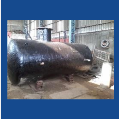
Underground Storage Tank
